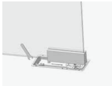
E. 利用配套工具，扭动地弹簧两侧的定位螺丝，进行左右微调； Using auxiliary tools, twist floor spring on either side of the positioning screw, about fine tuning;
