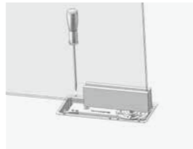
F. 利用螺丝刀，扭动地弹簧尾端的螺丝，进行上下微调； Using screwdriver, twist floor spring tail screws, carries on the fluctuation fine-tuning;
