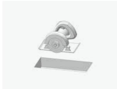
B. 使用切割机械，沿线切割出空位； Use along the cutting machine, cutting into space;
